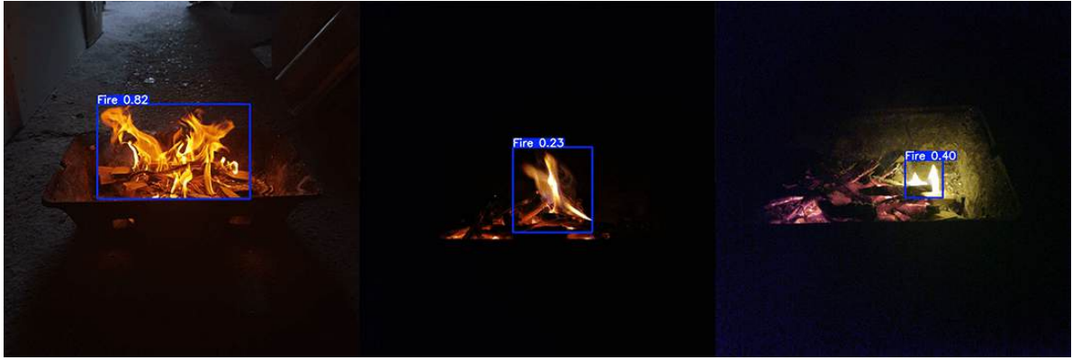
Figure 2.9: Visualization of object detection showing the detection and localization of fire within images.
