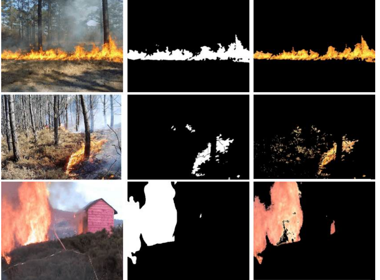
Figure 2.5: The visualization of using K-Means clustering to segment fire. Image source: Rudz et al. [59] .
